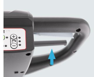
7. Adjust handle to fit different operators' height and then start cleaning by placing the hands on the safety switches
