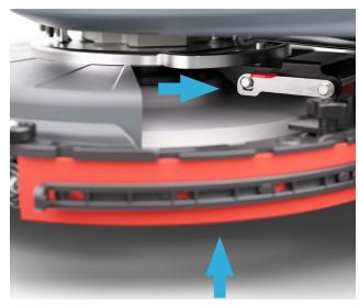
9. Lift the squeegee up by hand until it locks in up position and turn suction off for double scrubbing. To go back to working mode, use the red lever to release the squeegee. and turn suction on again.
