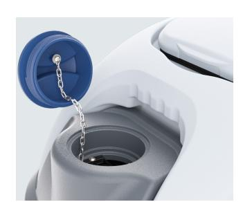
**5.** Remove the blue cover, fill the tank with clean water and use maximum temperature 40 degree. Add appropriate low foaming detergent according to dosage information.
