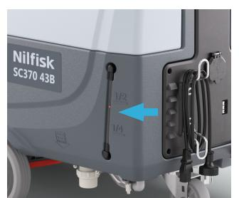
**6.** Check the solution level by the red ball on the left side of the machine.
