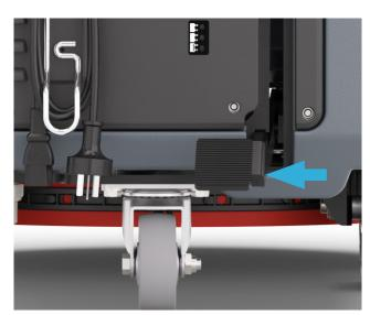
**2.** Lift the deck by pressing the pedal.
