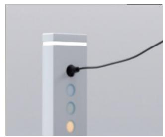
**18.** Daily: Charge the batteries: Connect the battery charger cable to the electrical socket. Light turns red when charging and green when the charging is complete.
