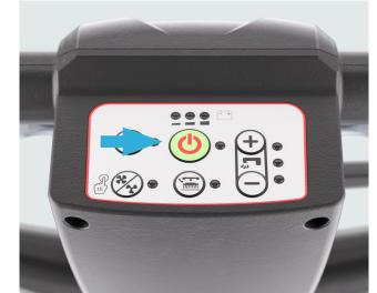
**4.** With the machine on, press one of the safety switches to engage the brush/pad-holder, then release it. If necessary, repeat the procedure until the brushes/pad-holder is engaged. The squeegee is raised and lowered with the deck.
