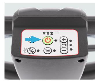
**10.** When scrubbing is complete, turn off the machine to perform the following maintenance
