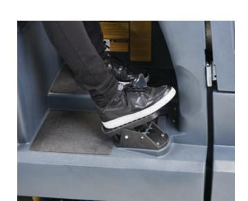
11. Press the forward pedal and start operating the machine
