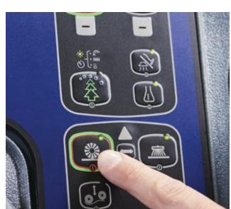
**4.** Adjust main broom pattern per operators manual to avoid overload condition. Inspect broom and drive for debris or adjust height if overload detected
