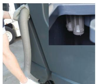
**4.** Squeegee hose free from debris. Verify recovery tank is not full and float balls are blocking motor inlet
