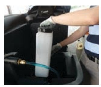
**3.** Fill the EcoFlex<sup>™</sup> tank (placed under the seat) with a detergent suitable for the work to be performed (highly concentrated detergent)
