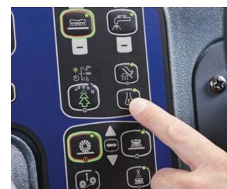
10. Adjust to the desired chemical concentration (shown in the display)
