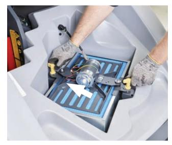
16. Dump the hopper, remove and clean the filter
