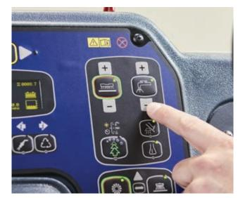
**9.** Adjust to the desired water flow
