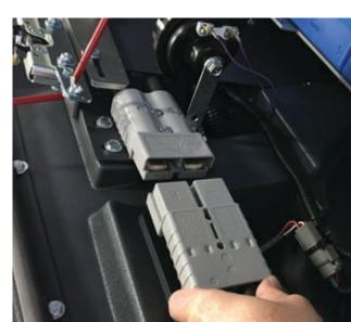
2. For the battery version check the battery voltage and if needed recharge
