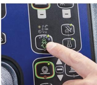
**12.** Press the Ecoflex<sup>™</sup> switch whenever you temporarily need a greater cleaning power
