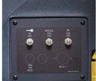
**4.** Inspect the circuit breakers
